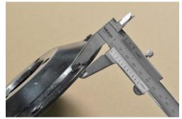
Measure the thickness of the inner ring
