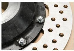
... > Flat washer > Nut. Torque tighten the nut to 6 Nm.
