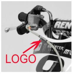
Tightening torque of banjo-bolt on Moto-Master radial master cylinder: 15 Nm Tightening torque of banjo-bolt on Moto-Master Supermoto race caliper: 17 Nm (bleed valve 10 Nm) Tightening torque of banjo-bolt on standard OEM caliper: may vary according to make and model of the bike, please consult bike manufacturer's user's guide for exact specification. Filling/bleeding of the brake system: consult master cylinder mounting & safety instructions.
