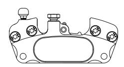
Tightening torque mounting bolts caliper-adapter: 22Nm
