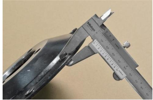
Measure the thickness of the inner ring
