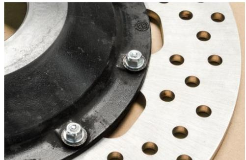
... > Flat washer > Nut. Torque tighten the nut to 6 Nm.
