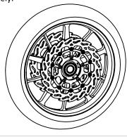
\*\*\*Make sure the turning direction of the wheel and brake discs is correct!
