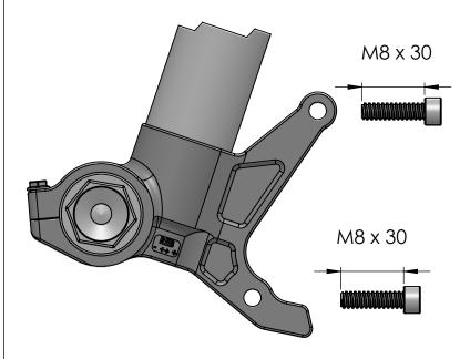
Use the included Moto-Master M8 x 30 mm bolts to mount the caliper adapter bracket.
