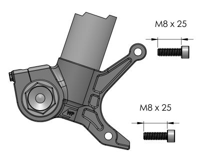
Use the included Moto-Master M8 x 25 mm bolts to mount the caliper adapter bracket.
