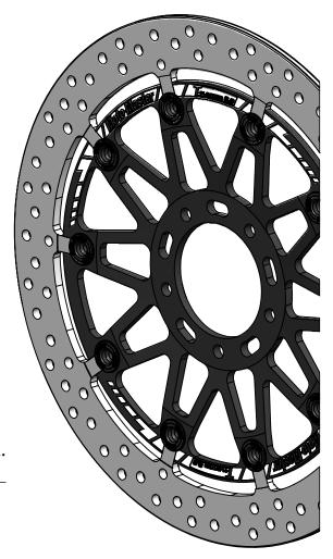
Make sure to check the amount of free play between the aluminium inner carrier and the stainless steel T-pin before every ride.
